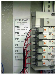
Figure 1.2 50 Million Cycle Valves. An LTU8000H installation typically has to do over 10 million cycles per year!
