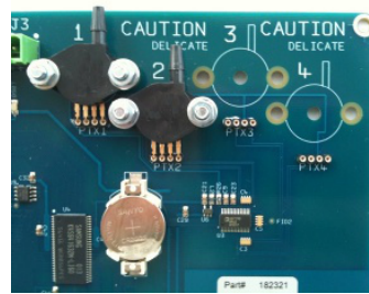
1-2 Channels on the same Circuit Board
