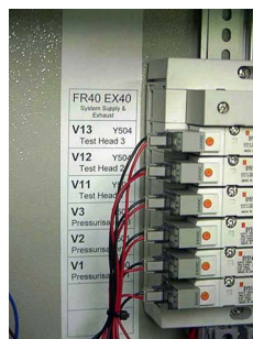
Figure 1.1 50 Million Cycle Valves. An LTU6000 installation typically has to do over 10 million cycles per year!
